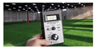
An ionization meter (above) measures levels to ensure there is an adequate number of positive and negative ions in the air to capture and destroy microscopic pathogens as well as pollen, dust, mold, VOCs, and odors.
