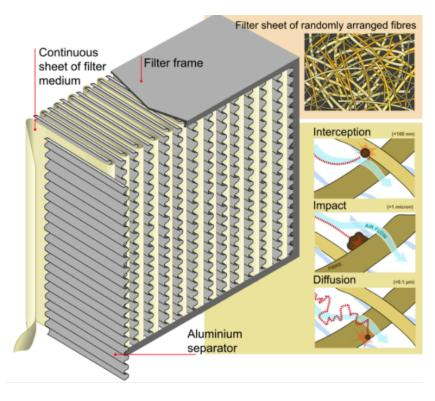
even better. A HEPA filter is not like a typical air filter, having considerable thickness of multiple mats of fibers randomly arranged to help catch a variety of particle sizes.
