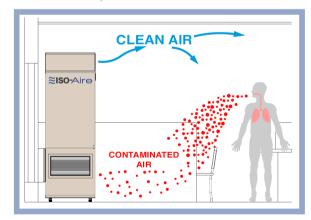
ISO-Aire pulls airborne contaminants away from the source and into the air purifier where they are captured and destroyed with a combination of medical-grade HEPA filtration, UVC, and/or ozone-free bipolar ionization.
