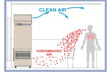
Our signature strategy to maximize safe and continuous air flow involves pulling air and airborne contaminants away from the source utilizing a high-powered fan. Recirculation models continuously capture and destroy harmful aerosolized particles and return purified air into the building environment.
