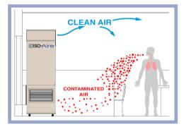
ISO-Aire pulls airborne contaminants away from the source and into the air purifier where they are captured and destroyed with a combination of medicalgrade HEPA filtration, UVC, and/or ozone-free bipolar ionization.
